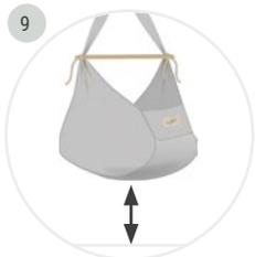
Check the correct height as described in the following point. The distance between the floor and the spring cradle must be between 50 and 60 cm when empty.
